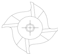
Non Centre Cutting
