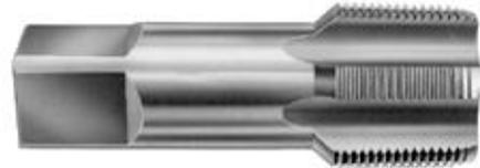
Ideally the hole should be reamed first before using a tapered tap but often is not. The result is that only the first 3 threads are formed to full profile.
