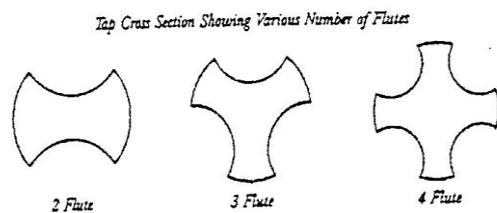
The flutes are grooves which run along the body of a tap. These flutes can be milled (as in carbon steel taps) or more generally ground (as in High Speed Steel). They provide a path for chip removal and also to carry cutting fluid to the front of the tap.
