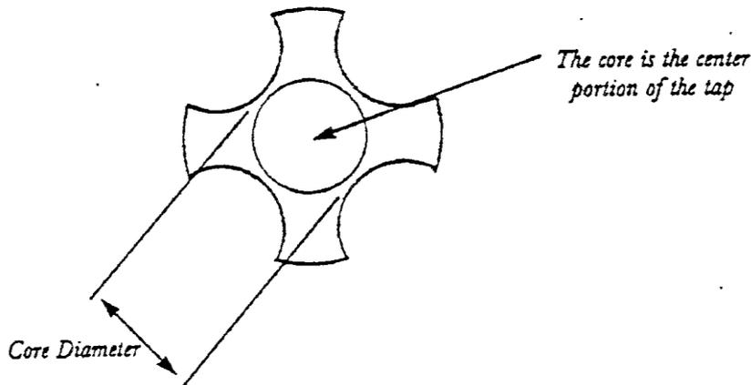
The core is the centre portion of the tap that separates the flutes. This provides the strength of the tap. As the number of flutes increases, the core becomes larger, increasing the strength of the tap.
