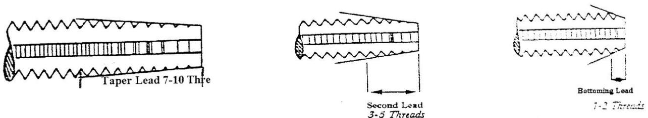
There are three standard leads used on taps:- Taper, Second & Bottom.
