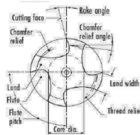
The body of the tap is made up of flutes, land, core, diameter, thread lengths and lead. These elements of the body portion produce the threaded hole.
