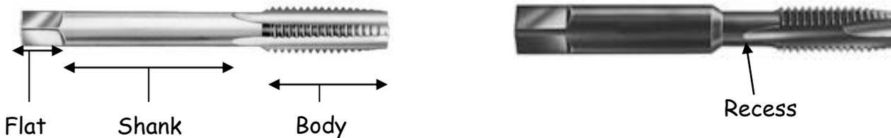
The shank is the part of the tap that fits in to the tap holder. The end of the shank is made square for driving and rotating the tap. The surfaces of the square are known as the "flats"
